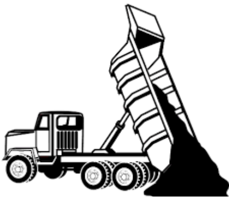
Before dumping, verify that the load has not SHIFTED in transit.
