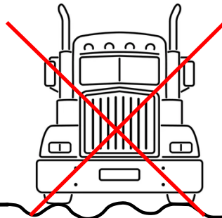
Soft Ground UNSAFE
